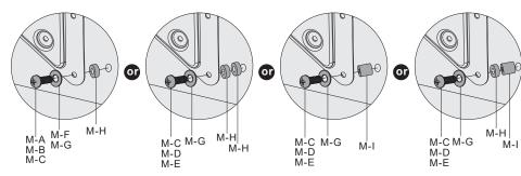
Note: Choose the appropriate screws, washers and spacers (if necessary) according to the type of screen.
