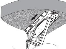
Hang the ceiling mount so that the screws fit into the keyhole openings. Slide slightly the ceiling mount into place and then tighten the screws.
